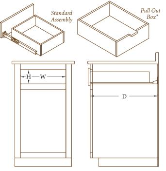
**STANDARD BOX** is 1/2" Baltic Birch sides with butt joints and 1/4" Luan bottom
